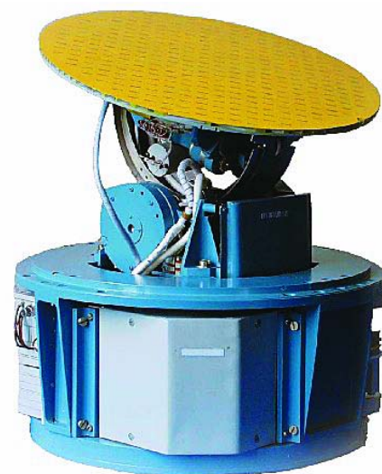
Upgraded 9B-1103M active radar homing head (diameter 350 mm)
